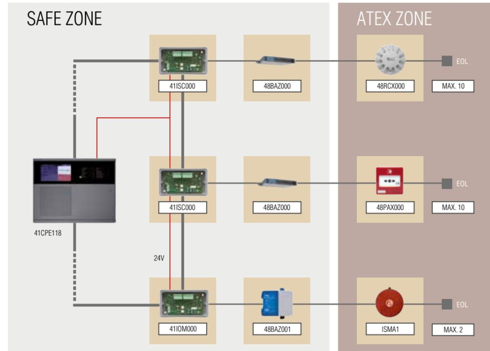
**EXAMPLE OF ATEX CONNECTION TO A CONVENTIONAL CONTROL PANEL**
