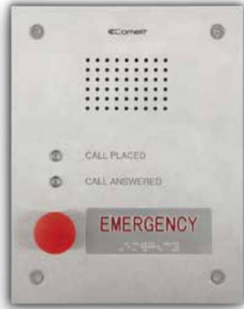
Stainless steel panel with a single call button and indicator LEDs for call forwarded and call answered. Complete with audio module art. 1682 for ViP system and flush-mounted box. "EMERGENCY" model with Braille text. Can also be surface mounted with accessory art. 3461, available to purchase separately.
