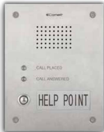
Stainless steel panel with a single call button and indicator LEDs for call forwarded and call answered. Complete with POE audio module for ViP system and flush-mounted box. "HELP POINT" model. Can be wall-mounted using accessory art. 3461. Panel dimensions: (L x H x D): 180 x 229 x 3 mm.
