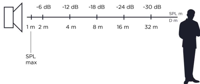
As you can see from the above image, the sound level produced by a speaker decreases as the distance from the listening point increases. If the consumption due to the environment is not taken into account, we can see that as the distance doubles this contributes to a weakening of -6 dB in the sound pressure level.
