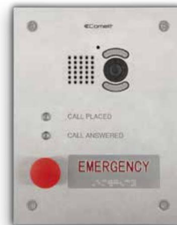
Stainless steel panel with a single call button and indicator LEDs for call forwarded and call answered. Complete with POE audio/video module for ViP system and flush-mounted box. "EMERGENCY" model with Braille text. Can be wall-mounted using accessory art. 3461. The panel is POE. Compatible with H.264 video format. Dimensions 228.6x177.8x3 mm.
