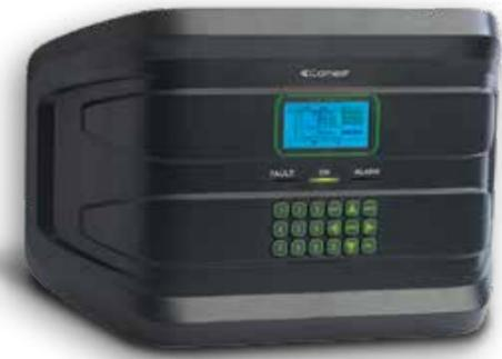
The wall-mounted gas control panel art. 47CPG424 can manage up to 4, 8, 16 or 24 remote gas detectors. The backlit colour graphic display (RGB) on the front of the control panel can be used to view the values of all gas detectors connected to it in real time. Equipped with 4 inputs and 5 relay outputs, which can be expanded up to 24 detectors and 25 relays using the relevant expansion boards. Power supply voltage 230 Vac.
