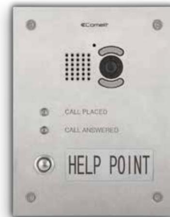
Stainless steel panel with a single call button and indicator LEDs for call forwarded and call answered. Complete with POE audio/video module for ViP system and flush-mounted box. "HELP POINT" model. Can be wall-mounted using accessory Art. 3461. The panel is POE. Compatible with H.264 video format. Dimensions 228.6x177.8x3 mm.
