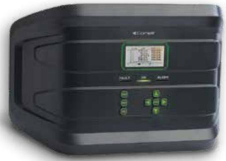
The wall-mounted gas control panel art. 47CPG408 can manage up to 4 or 8 remote gas detectors. The backlit graphic display on the front of the control panel can be used to view the values of all gas detectors connected to it in real time. Equipped with 4 inputs and 5 relay outputs, which can be expanded up to 8 detectors and 9 relays using the relevant expansion boards. Power supply voltage 230 Vac.
